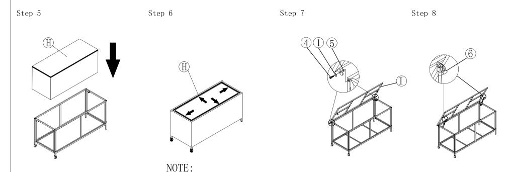
DO not tighten screws completely until assembling is completed
